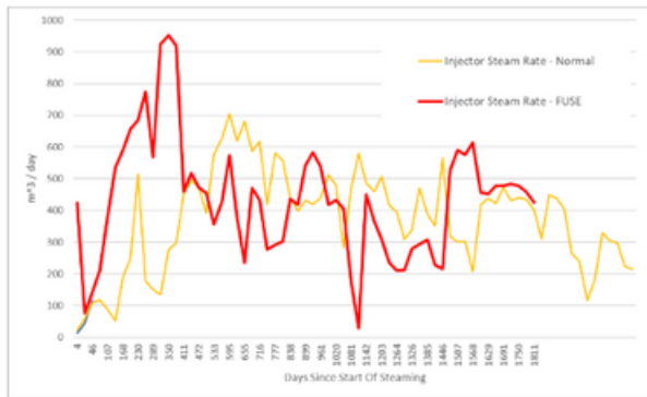
Figure 3b: More steam can be injected when the injector is stimulated by FUSE as compared to the normal circulation start-up well.
