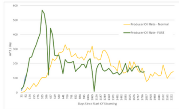
Figure 3c: More oil is produced when the SAGD well pair is stimulated by FUSE as compared to the normal circulation start-up well.
