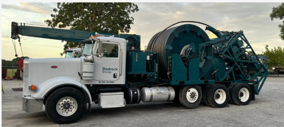
Figure 3 - Example of a coiled tubing platform for shallow geo-field construction of large buildings in dense urban areas (Torres et al. 2024).
